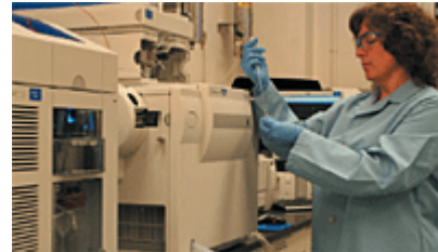
A Pacific Northwest National Laboratory (PNNL) scientist works on the capillary electrophoresis electrospray ionization ion trap mass spectrometer (CE/ESI/MS). This instrument is designed to efficiently separate and detect a range of analytes. (Source: PNNL)
